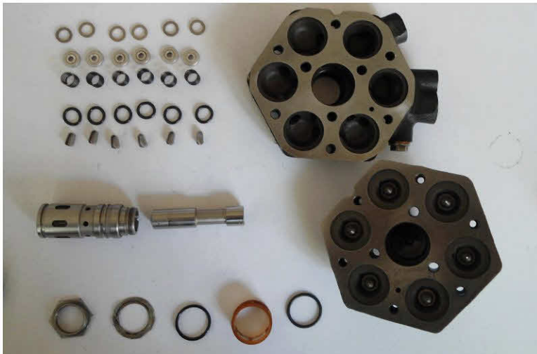
opened fuel distributor (picture taken of a 6 cylinder Porsche fuel distributor)
